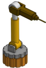
Fig. 2: CAD model of RRPR mechanism.
